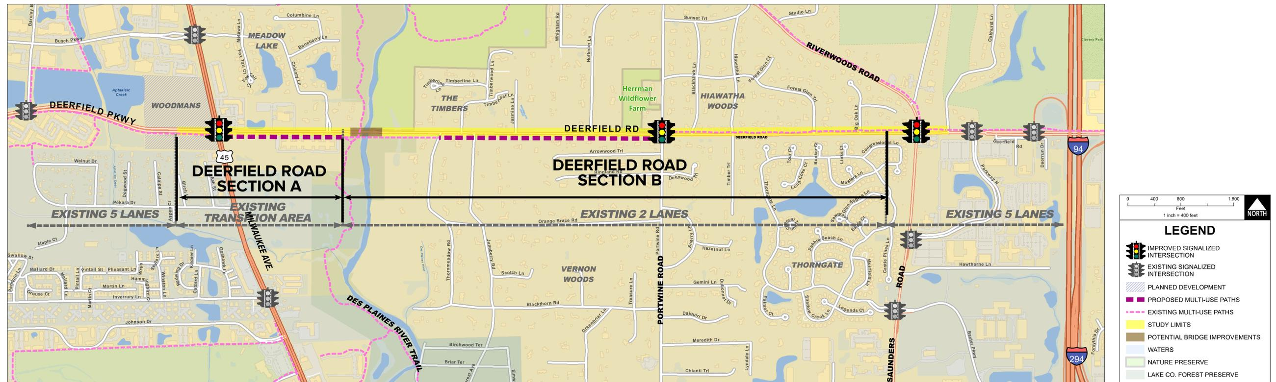
Due to different adjacent land use and transportation needs, the Deerfield Road corridor was broken up into two sections for alternatives development and evaluation, **Section A** consisting of improvements related to the Milwaukee Avenue intersection and **Section B** from the Milwaukee Avenue intersection improvement to Saunders/Riverwoods Road.
